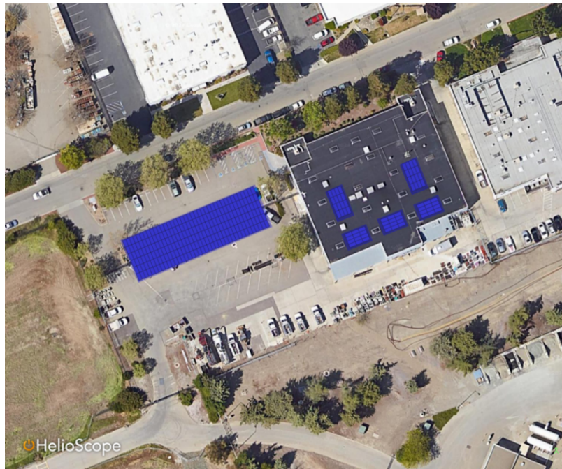
Figure 2 – Solar Layout at the Field Operations Facility
