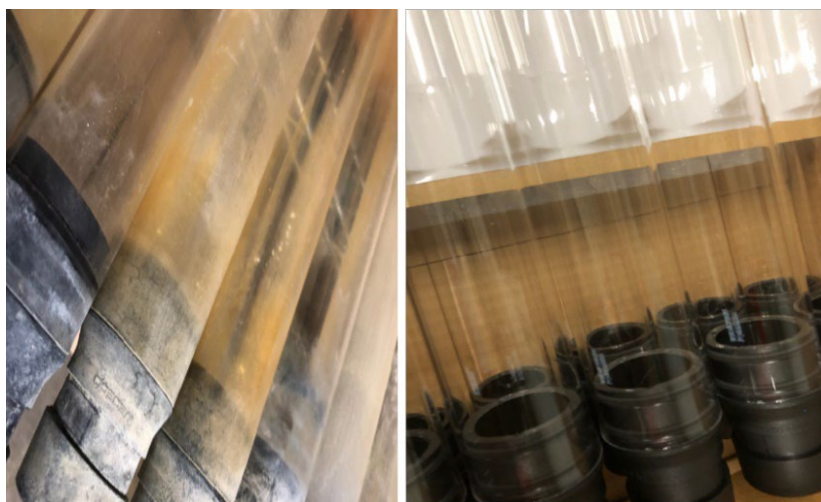
Photos: old quartz sleeves (left), new quartz sleeves (right)
