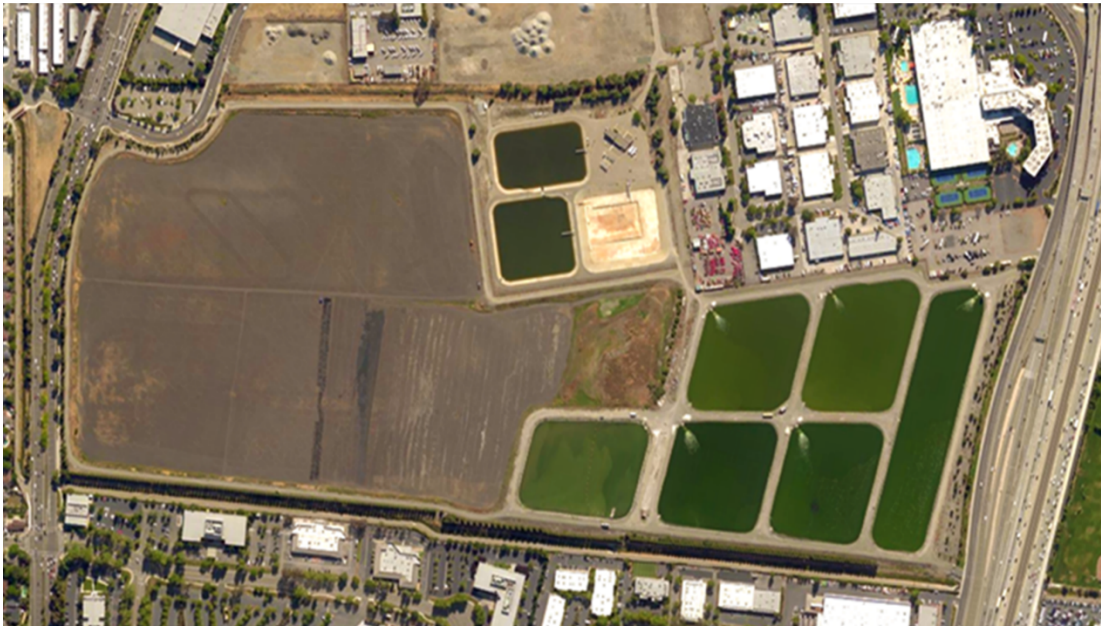
Figure 3 Dedicated Land Disposal Site (left) and Facultative Sludge Lagoons (right)
