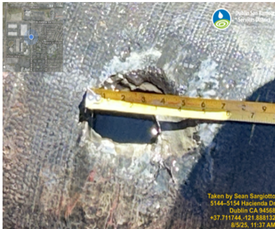
Photos: ( Left) Pipe break, (Right) Completed repair of 20-inch recycled water main using pipe provided by the City of Pleasanton.
